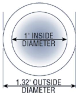
Slot spacing in illustration at right is exaggerated to show slot size in relation to AllVent pipe. For actual dimensions, refer to text description of product on page 25.
