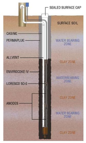
EnviroCoke IV in combination with PermaPlug provides total environmental control.
